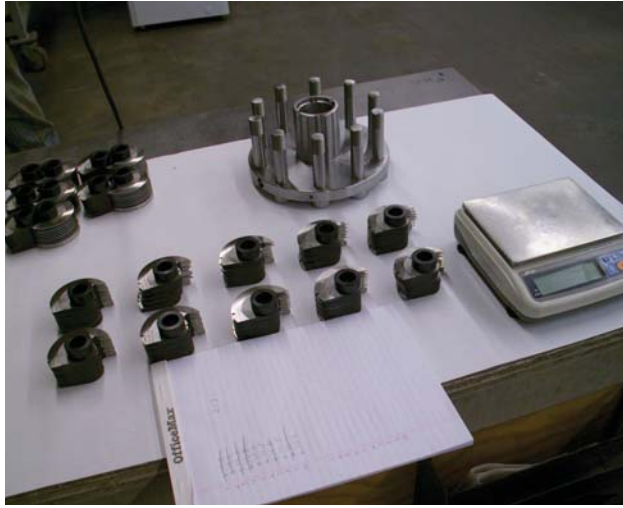
Cutter Stacks & Washers Balanced to 0.1 Gram
