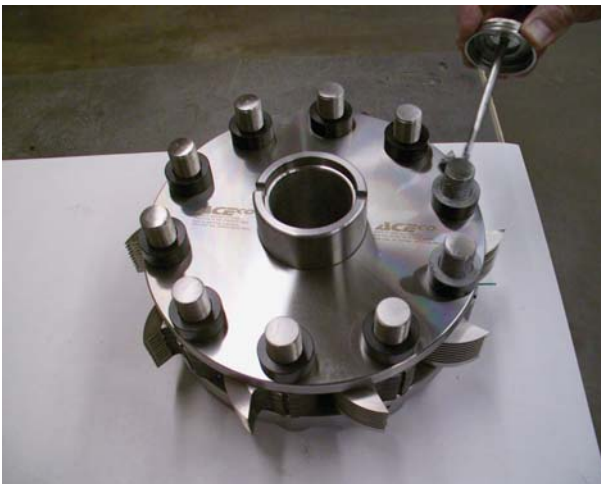
Anti-seize is applied to the bolt threads.
